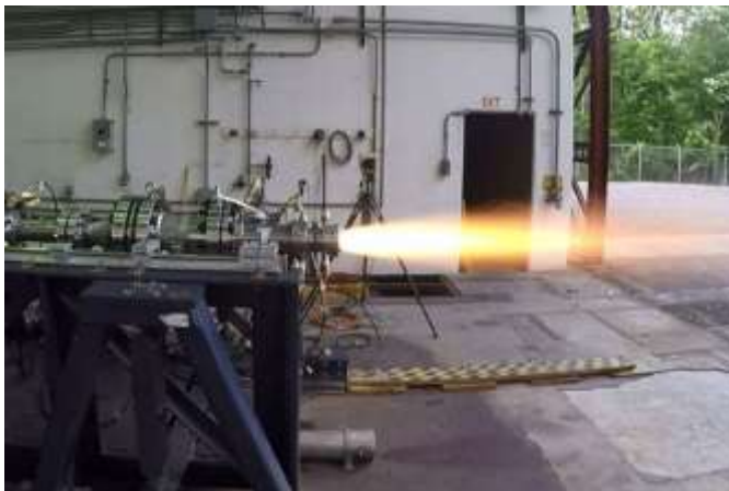
Test of Northrop Grumman's ramjet engine for extended-range 155 mm artillery shells
